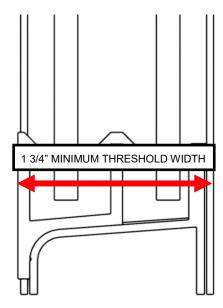
The unit requires 1 3/4" of threshold width to ensure the unit does not hang off of the edge. It is up to the installer to determine if the threshold is wide enough to drill into so as to not damage the finished surface. Please take appropriate precautions to be sure tile surfaces are wide enough so that they are not broken during the installation process.
