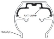
**7** This bath enclosure is equipped with safety tee-lock **Wall Jambs**. When installed properly, the header is permanently locked to the **Wall Jambs** and cannot be accidentally dislodged.
