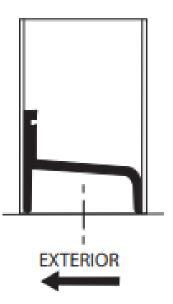
**3** Press both **Wall Jambs** (**SC896**) into position over the **Track**. Masking tape can be used to hold the parts in place temporarily.
