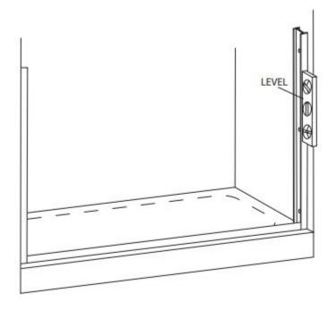
**4** Before replacing the **Track**, force a slight downward bow in the extrusion. This will ensure the track fits tight to the threshold.
