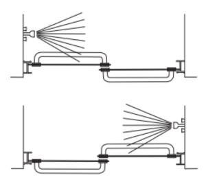
12 Lift the Inner Panel into position with the Rollers engaging the groove in the Header. Repeat for the Outer Panel.
