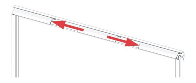
9 If not installed from the factory, install the **Hanger Brackets (SC8240)** onto the glass. Install the **Roller (SC4082)** and the **Roller Screw (SCR44)** on each **Hanger Bracket**.
