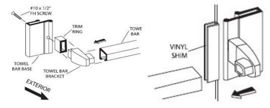
11 At the center of the Inner Panel, press the (2) Pull Handles (SC4129) and (2) Vinyl Shims (SCV294) into place on each edge of the glass.
