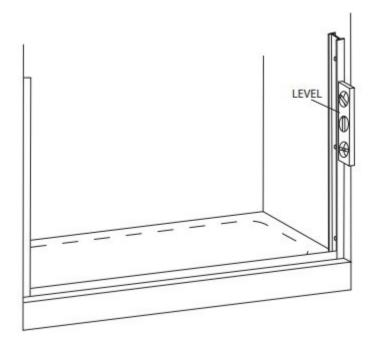
**4** Before replacing the **Track**, force a slight downward bow in the extrusion. This will ensure the track fits tight to the threshold.
