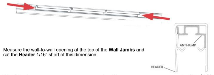
**7** This bath enclosure is equipped with safety tee-lock **Wall Jambs**. When installed properly, the header is permanently locked to the **Wall Jambs** and cannot be accidentally dislodged.
