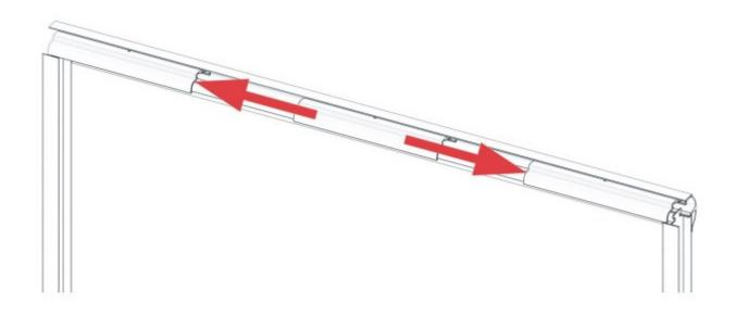
**9** If not installed from the factory, slide and install the **Hanger Brackets (SC8239)** onto the glass. Tighten the three screws on each bracket evenly to securely grip the glass panel.
