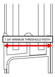
The unit requires 1 3/4" of threshold width to ensure the unit does not hang off of the edge. It is up to the installer to determine if the threshold is wide enough to drill into so as to not damage the finished surface. Please take appropriate precautions to be sure tile surfaces are wide enough so that they are not broken during the installation process.
