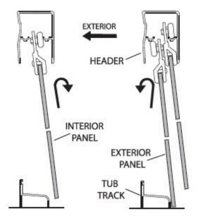
**NOTE:** Panels will need to be close to the center of the opening in order to be installed. If there is ever reason to remove the panel, the panel will again need to be centered in the opening to avoid the **Anti-Jump Rails**.
