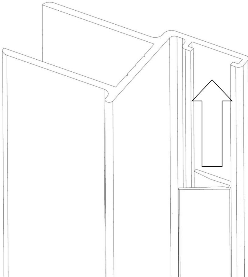
**22** Slide the **SC552 Strike Jamb [5]** over the **SC508 Wall Jamb [4]**. Fully compress the jambs.
