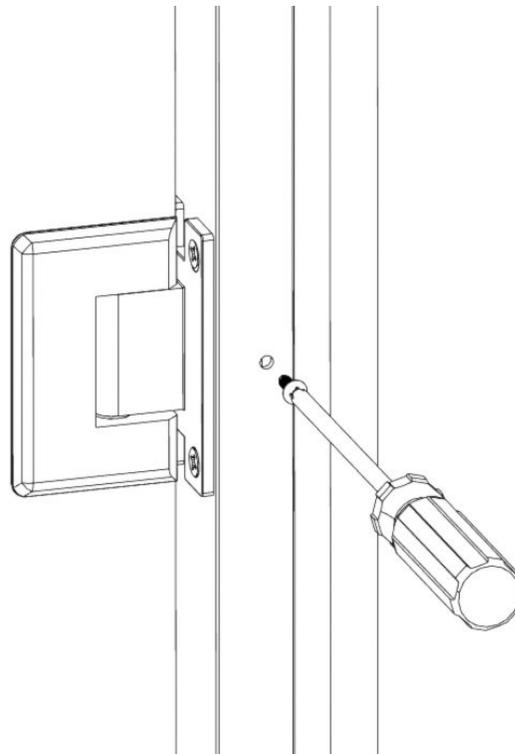
**20** After all 4 **Hinge Jamb Screws [11]** are installed, remove the 7/16" shims and carefully open the door, making sure the glass does not contact anything.
