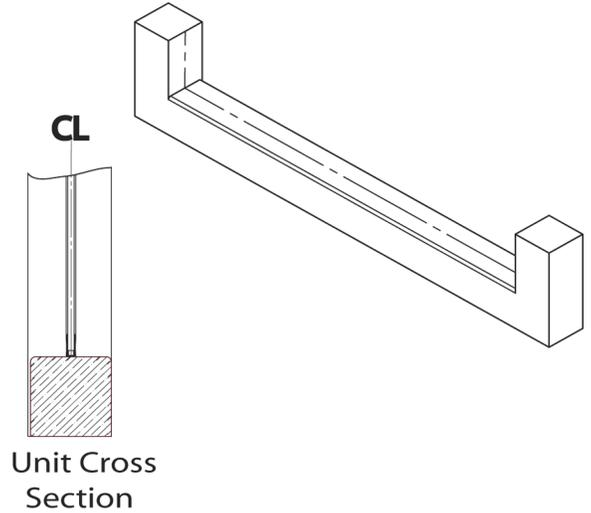
*Centerline (CL) is a term used to describe the center or mid-point of the unit. The most common unit centerline position is the middle of the threshold. CL is marked in when visible in images.*
