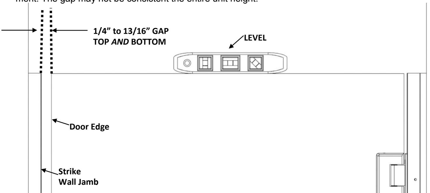
**18** While keeping the door level, plumb, and with the correct gap at the strike side; drill 5/32" holes through the **SC982 Wall Jamb [2]** at the locations marked by the holes near each hinge in **SC983 Adjustable Jamb [3]**. The holes are on the side of the jamb, both inside and outside of the shower.
