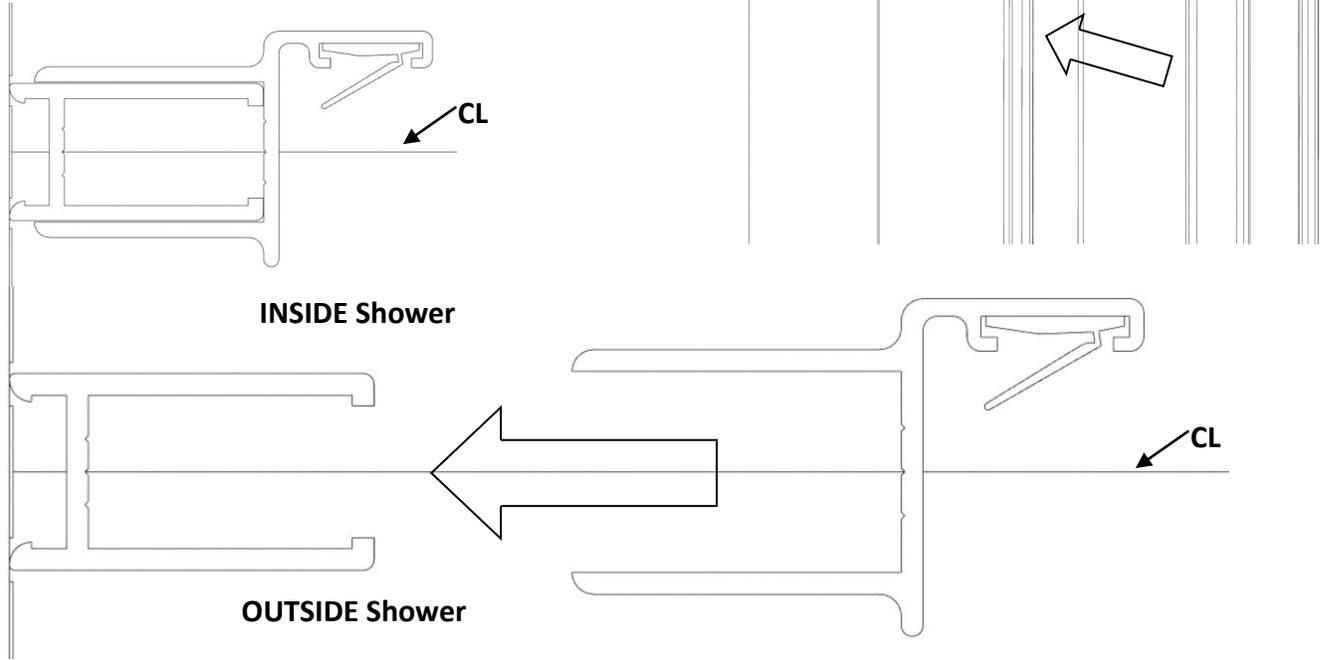
**23** Close the door against the **SC552 Strike Jamb [5]**. Slide the **SC552 Strike Jamb [5]** over towards the door, leaving a consistent 3/16" gap between the glass and the jamb.
