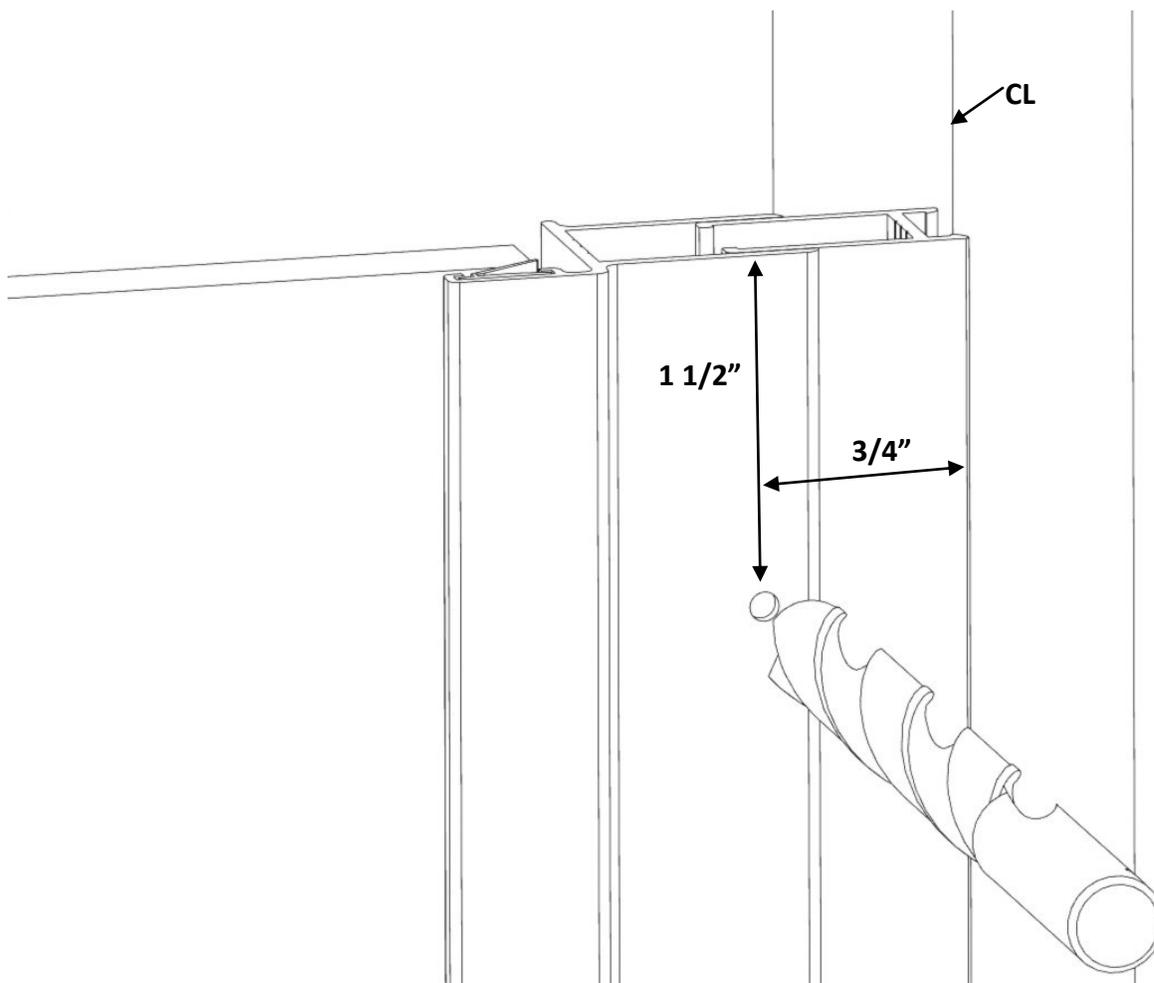
Insert screw **SCR24 [13]** into each hole to secure the strike jamb into position.
