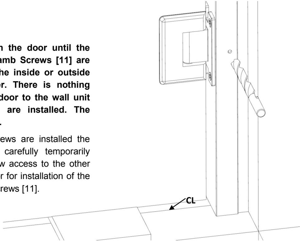
**19** Insert **Hinge Jamb Screws [11]** into each hole drilled in step 18.
