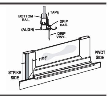
Adjust the drip vinyl [W] by sliding it left or right until it just touches the curb. Trim the vinyl (flush with the pivot end and notch ¼" longer than the drip rail as shown on the strike end). Secure it with one #6 x 3/8" truss head screw [E] in the pivot end of the drip rail.
