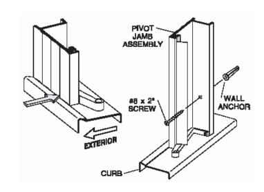
Replace the pivot jamb and attach to the wall with three #8 x 2" truss head screws [J].
