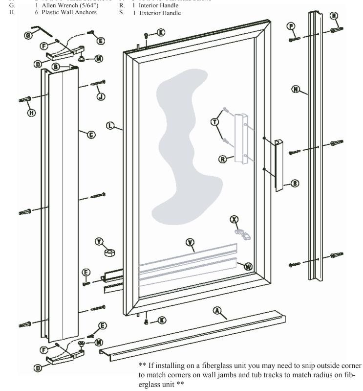
The Framed Pivot Shower Door is completely reversible and may be installed pivot-right or pivot-left. Using the diagram, determine the correct position for your installation. For maximum waterproofing, the pivot jamb should always be opposite the shower head. These instructions depict a pivot left installation.
