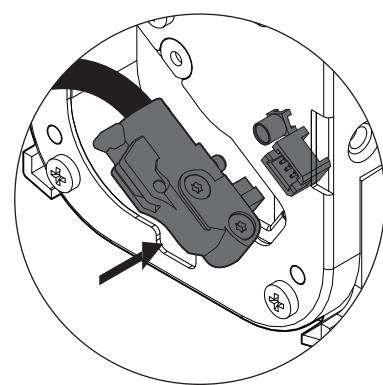
If connector lever is extended, push it down.
