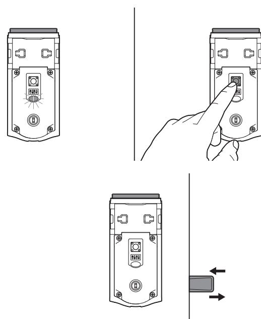
If the latch bolt does not retract and extend on its own: remove battery pack, wait 15 seconds, and attempt the process again.
