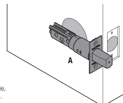
b If the latch holes are centered in the door hole, no adjustment is required. Proceed to step 4.
