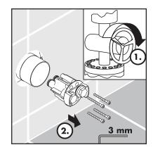
• Cut the plaster shield 1/16" from the surface of the finished wall.
