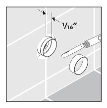
• Install the sealing rings and sleeve. The screws require a 3 allen wrench (included).
