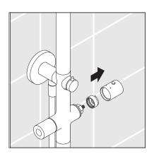
• Divert the water to the handshower. Turn on the water with the volume control. Place a thermometer in the water stream. Turn the thermostatic mixer valve stem until the water is 100°F.
