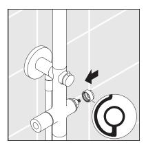
• Replace the handle with the red safety stop override button at the 12:00 position. Tighten the handle screw.
