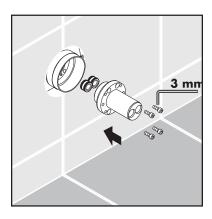
• Seal the wall around the rough with a non-staining waterproof bathroom sealant suitable for the wall surface
