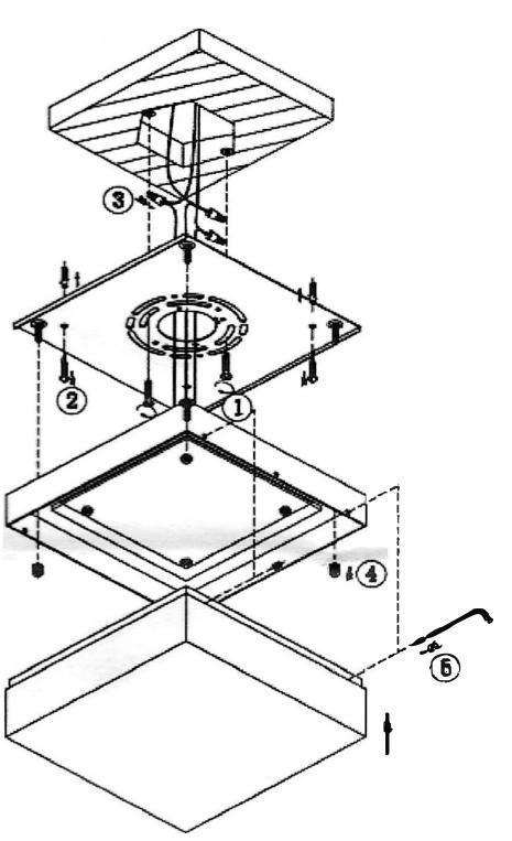
A:Copper ground wire to ground wire-if you only have two wires coming from the electrical box, connect the fixture's copper wire to the green ground screw on the mounting plate.
