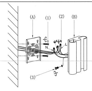
To prevent moisture from entering the outlet box and causing a short, seal around the top and side perimeter between the fixture and the wall surface with weather resistant caulking (see illustration a).
