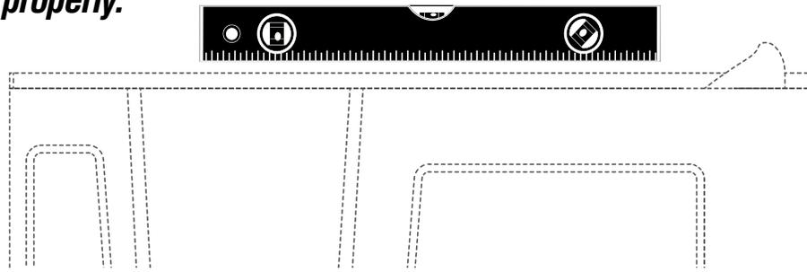
***Adjust leveling feet as needed making sure all feet are completely touching the floor. The tub must be completely level to avoid leakage.***
