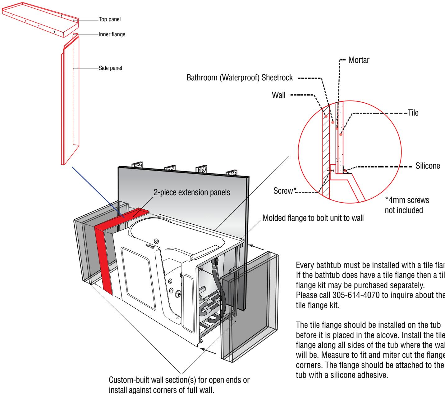
Every bathtub must be installed with a tile flange. If the bathtub does not have a tile flange then a tile flange kit may be purchased separately. Please call 305-614-4070 to inquire about the tile flange kit.
