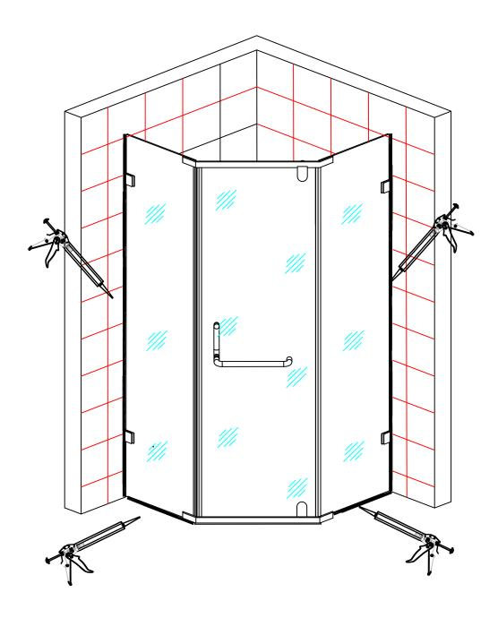
Using bathroom rated silicone sealant or caulk, seal the bottom each fixed glass panels to shower floor. Seal along each edge of fixed glass panels where the wall and fixed glass panels meet.
