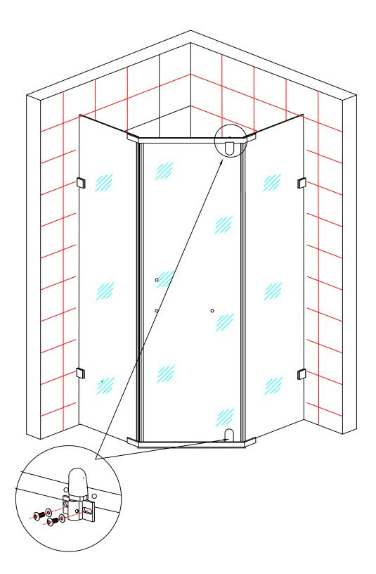
Using the hardware provided install the hinges onto the mounting cross bars.
