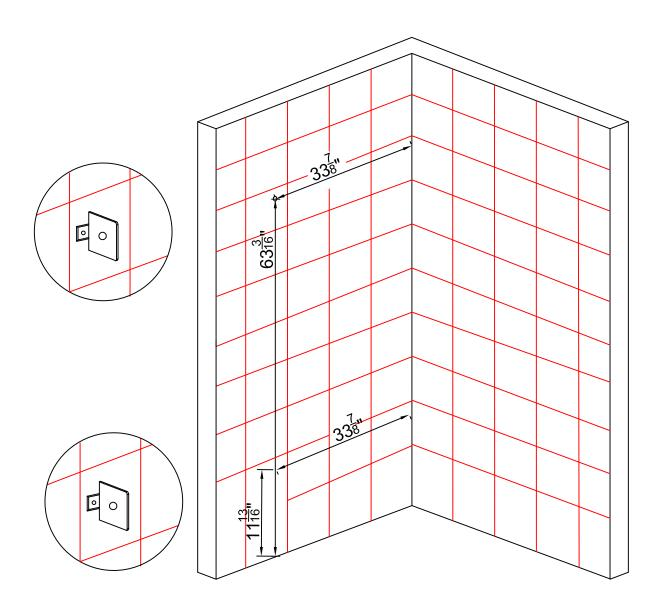
Install all of the wall material or materials you intend to use before installing the wall channels this includes all moisture resistant wall board or rock board, tile, stone or other wall covering.
