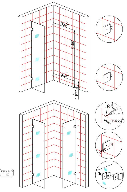
Using screw pack (2) attach the glass clamp to wall using M4x40 screws. The glass clamp should be postioned so that single hole is facing toward the inside of shower.
