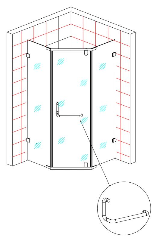
Install the door handle using the hardware provided be sure to use the silicone washer provided between the glass and the door handle to prevent scratching.
