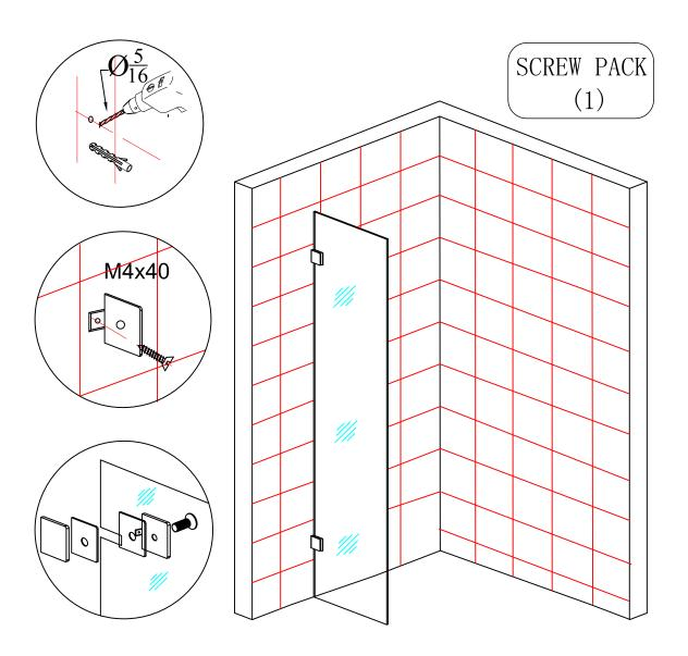
Using the appropriate drill bit for your wall surface drill each hole location with a 5/16" diameter drill bit. Install the plastic wall anchors provided into the drilled holes
