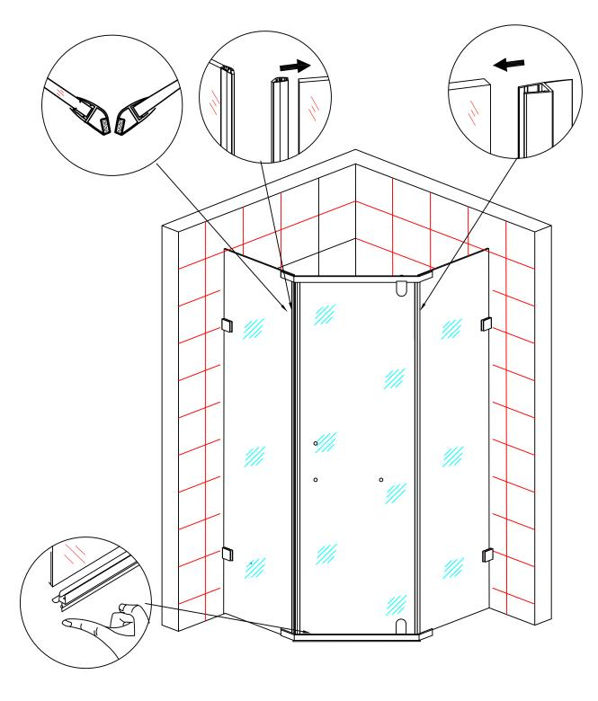
Install the bottom seal and the side magnet seals onto the door and fixed glass. Once you have installed all of the seals close to door and ensure a seal is created the entire length of the door. Make adjustments if necessary to the door to create a positive seal.
