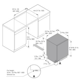
$\mbox{\ensuremath{\mbox{\$}}}$  Flexible side trims (width without side trims: 23  $\%\mbox{\ensuremath{\mbox{\$}}}_{6}$  / 596)
