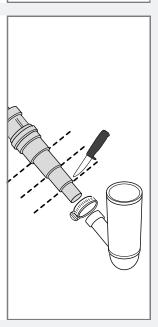
The drain hose can also be connected to a connection nipple on the sink unit's water trap. The connection nipple must have an internal diameter of at least 1/2".
