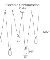
The three intermediate metal caps\* are adjustable to any point between the pendants to their immediate left or right.
