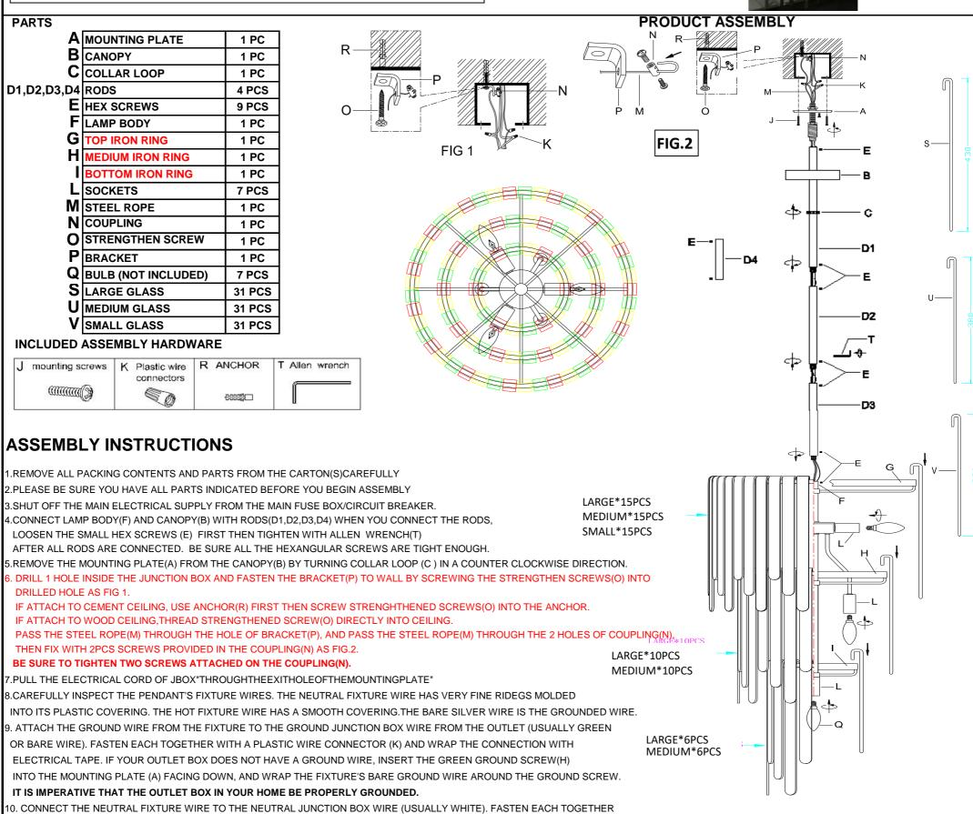
0. CONNECT THE NEUTRAL FIXTURE WIRE TO THE NEUTRAL JUNCTION BOX WIRE (USUALLY WHITE). FASTEN EACH TOGETHEF WITH A WIRE CONNECTOR (K) AND WRAP THE CONNECTION WITH ELECTRICAL TAPE. BE SURE NO STRANDS ARE EXPOSED.
