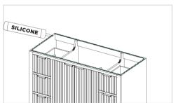
**STEP 7 -** PREPARE BASE CABINET Using a caulking gun, apply silicone around the top of the base cabinet.
