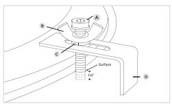
STEP 5 - ATTACH UNDERMOUNT CLIPS Please tighten Bolt (A) into wing nut (B) slide on washer (C) and guide through Under-mount clip (D) opening into threaded bolt hole in the countertop. ONLY-Hand Tighten Bolt (A) to a depth of about 1/4" below countertop surface. Then secure the Sink with the under-mount clip (D) by Tightening wing nut (B) only
