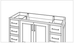
**STEP 6 -** ATTACH BASE CABINET TO WALL Place cabinet in desired location and determine where the wall study are.
