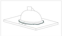
**STEP 4 -** DRY & SET Press down on the sink basin to seal the silicone. Remove any excess. Follow dry time recommendation found on your product, typically 12 to 24 hours.
