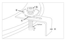
STEP 5 - ATTACH UNDERMOUNT CLIPS
