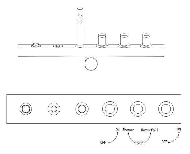
1. The middle faucet is functional faucet. The faucet is closed when it keeps in the middle position. When you rotate the faucet  $90^{\circ}$  to the left, the water will come out from the hand shower; and when you rotate the faucet  $90^{\circ}$  to the right, the water will come out from the waterfall.
