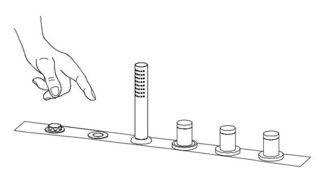
Press the on/off button at the first time to operate the bubble function; and press it by the second time to turn off the bubble function.
