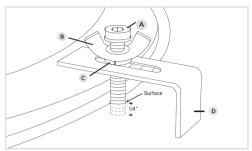
STEP 5 - ATTACH UNDERMOUNT CLIPS
