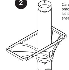
Carefully slide the plastic bracket over the top post and let it rest on the heads of the sheet metal screws.
