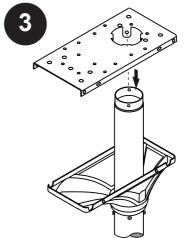
Attach the mounting plate to the post using the 4 small hex bolts, nuts and 8 small washers.
