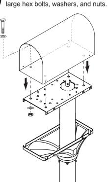
Once the mailbox is mounted, carefully push the plastic bracket up into the mailbox plate. Press the sides of the bracket inward making sure the four studs snap into the rectangular notches on the sides of the mounting plate as shown below.
