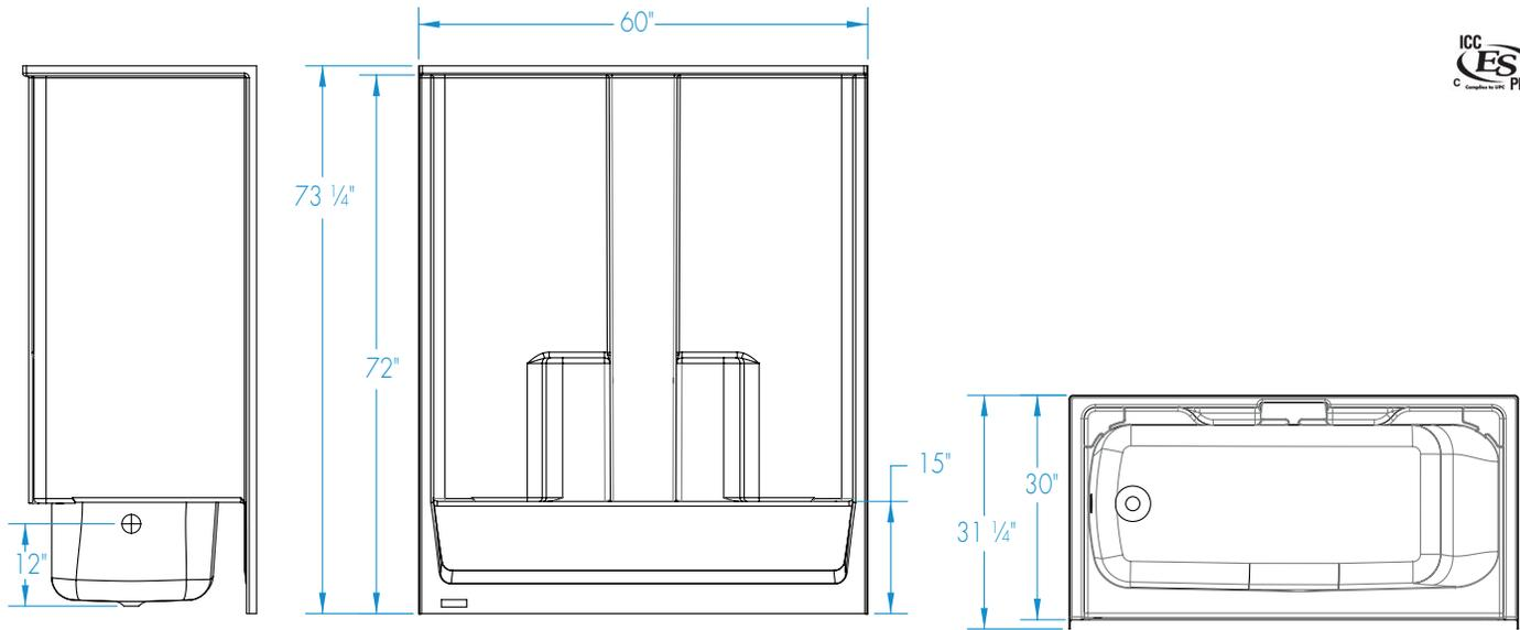
**FEATURES** lbs      Dimensional Tolerance  $\pm 3/8"$ . Dimensions needed for site preparation should be measured from the unit. Aquatic assumes no responsibility for preparatory work.
