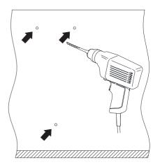
If screw locations are in wall stud, drive mounting screws directly into stud. If screw locations are not in stud. Drilling three 0.24"(6mm) diameter holes on the wall. Insert the plastic anchors into the holes and then drive screws into wall anchors.
