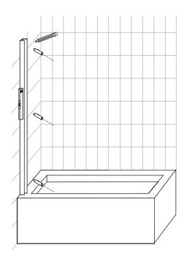
The profile must be checked with the spirit level whilst marking.
