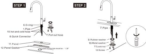
1. Position the faucet, deck plate and o-ring on the installation surface. And then put the faucet into center hole.
