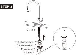
2. Adjust the position of the faucet and secure it with the fixing kit as photo.
