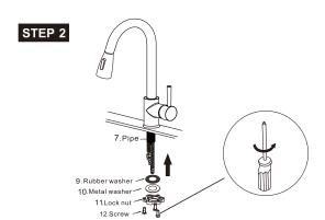
2.Adjust the position of the faucet and secure it with the fixing kit as photo.
