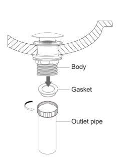
3. Install the pipe with the gasket inside.
