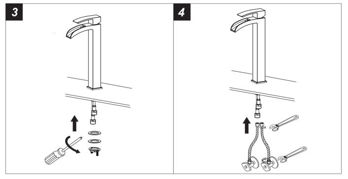
3. Place washer (16),metal gasket (17) over the shank under the sink. Install the locknut (18) and hand tighten it, then secure the faucet by tightening the screws of the locknut (18).
