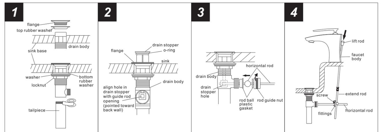
1. Remove pop-up drain stopper, and flange with top rubber washer for pop-up assembly. Insert drain body from underneath of sink drain hole. Replace flange and top rubber washer back to drain body. Tighten flange as far as possible. Remove and put silicone along bottom of. (Optional) Slide bottom rubber washer on drain body up against bottom of sink. Tighten washer and locknut firmly against base for tight seal. Remove tailpiece from drain body, add Teflon tape, replace tailpiece.
