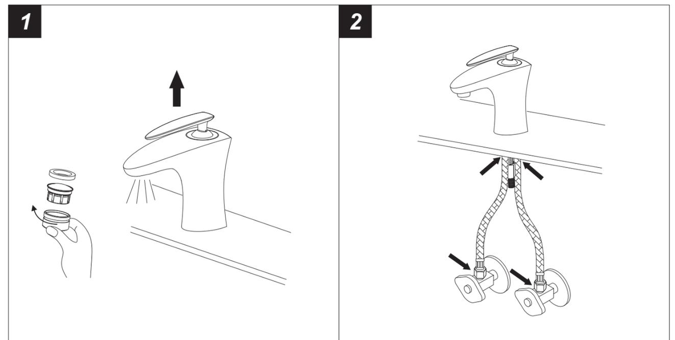
1. Remove the aerator by hand. Turn the faucet handle all the way on, turn on hot and cold water supply and flush water lines for one minute. Reinstall aerator by hand.
