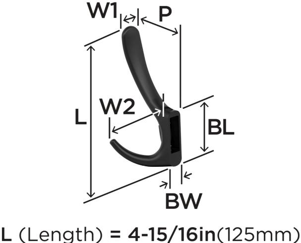
**P** (Projection) = **2-3/16in**(56mm) **BL** (Base Length) = **2-1/16in**(52mm)
