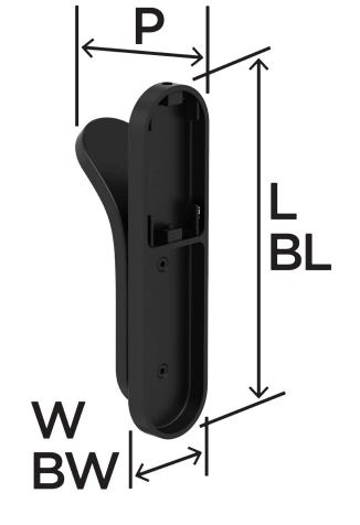
**W** (Width) = 1-5/16in(33mm) **P** (Projection) = 1-5/8in(41mm)
