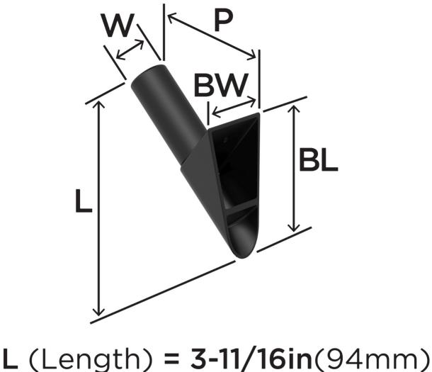
**BL** (Base Length) = 2-13/16in(71mm) **BW** (Base Width) = 1-7/16in(37mm)
