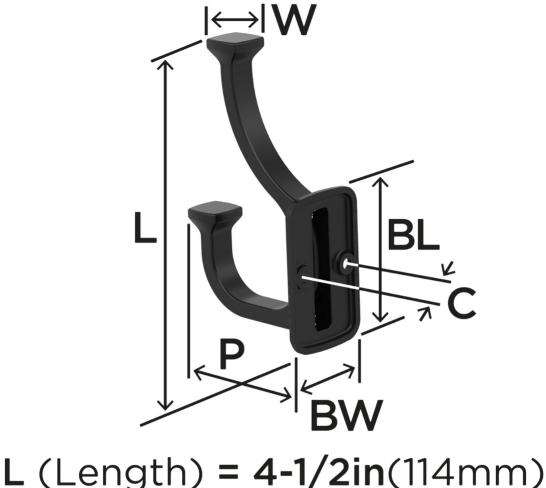
**W** (Width) = **11/16in**(17mm) **P** (Projection) = **2-5/8in**(67mm)
