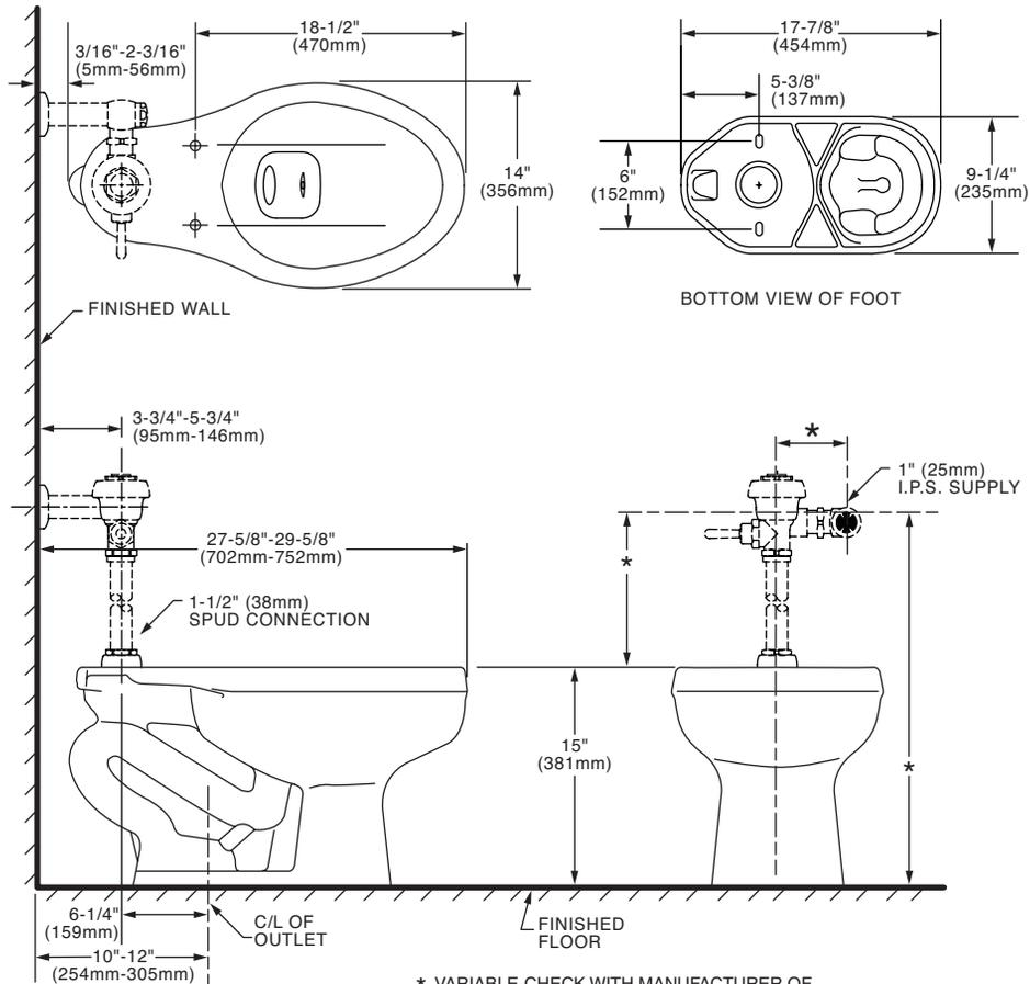
\* VARIABLE-CHECK WITH MANUFACTURER OF FLUSHVALVE FOR PROPER ROUGH-IN DIMENSIONS.
