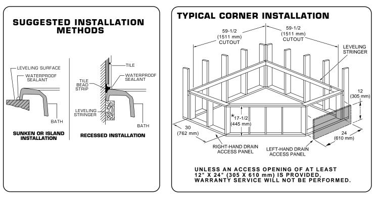
\* NOTE: If the optional apron (PN 0730.121) is to be used with this tub, the stringer height must be referenced from the finished floor.
