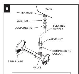
CAUTION: Overtightening of COUPLING NUT could result in breakage and potential flooding.
