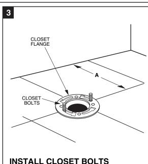
Install closet bolts in flange channel, turn 90°, and slide into place 6" (152 mm) apart and parallel to wall.
