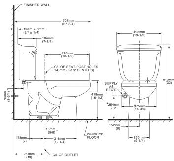
THIS TOILET IS DESIGNED TO ROUGH-IN AT A MINIMUM DIMENSION OF 254mm (10") FROM FINISHED WALL TO C/L OF OUTLET. SUPPLY NOT INCLUDED WITH FIXTURE AND MUST BE ORDERED SFPARATFI Y
