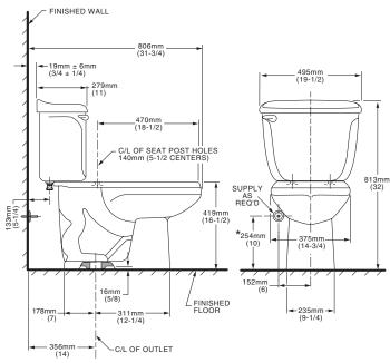
THIS TOILET IS DESIGNED TO ROUGH-IN AT A MINIMUM DIMENSION OF 356mm (14") FROM FINISHED WALL TO C/L OF OUTLET. SUPPLY NOT INCLUDED WITH FIXTURE AND MUST BE ORDERED **SEPARATELY**
