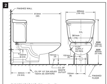
**DIMENSIONS (Nominal)** NOTE: Distance from floor to closet flange centerline (rough-in) must be 4" (102 mm) with flange surface flush to 1/16" (16mm) max. beyond finished wall.
