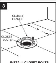
**INSTALL CLOSET BOLTS** Install closet bolts in flange channel, turn 90°, and slide into place 6" (152mm) apart and parallel to wall.
