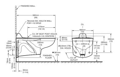
Toilet designed to meet ADA accessibility standards when top of seat height set at 432 to 483mm (17" to 19") from finished floor.
