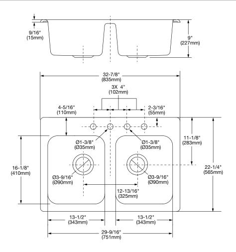
**NOTES:**\* DIMENSIONS SHOWN FOR LOCATION OF SUPPLIES AND "P" TRAP ARE SUGGESTED. FITTINGS NOT INCLUDED WITH FIXTURE AND MUST BE ORDERED SEPARATELY. SEALING COMPOUND SUPPLIED BY OTHERS.
