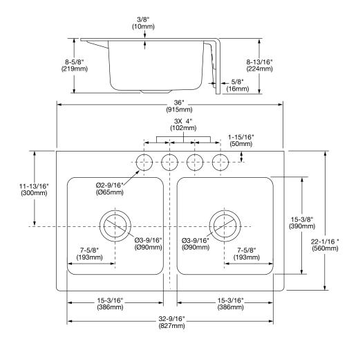
\*\*DIMENSIONS SHOWN FOR LOCATION OF SUPPLIES AND "P" TRAP ARE SUGGESTED. FITTINGS NOT INCLUDED WITH FIXTURE AND MUST BE ORDERED SEPARATELY. SEALING COMPOUND SUPPLIED BY OTHERS.
