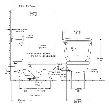
NOTES: THIS COMBINATION IS DESIGNED TO ROUGH-IN AT A MINIMUM DIMENSION OF 254mm (10) FROM FINISHED WALL TO C/L OF OUTLET.
