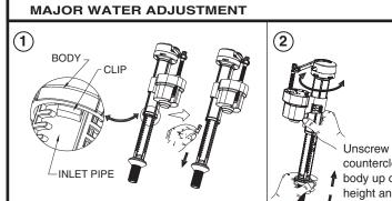
Unscrew the fill valve body counterclockwise, push the body up or down to the desired height and refasten valve body by turning clockwise.
