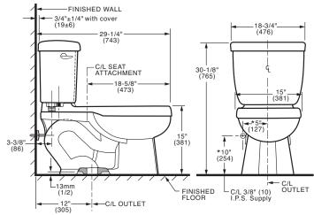
THIS TOILET IS DESIGNED TO ROUGH-IN AT A MINIMUM DIMENSION OF 305MM (12") FROM FINISHED WALL TO C/L OF OUTLET. SUPPLY NOT INCLUDED WITH FIXTURE AND MUST BE ORDERED SEPARATELY.
