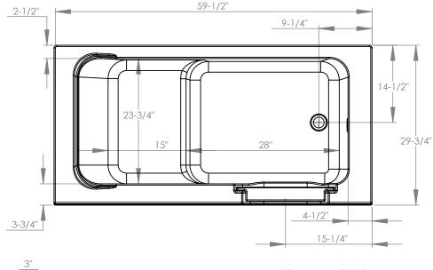
TUB IS SUPPORTED BY THE FRAME AND FIVE INTEGRATED ADJUSTABLE FEET, NO ADDITIONAL SUPPORT IS REQUIRED.
