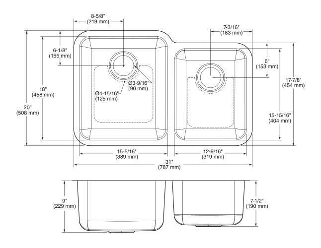
**NOTES:**\* DIMENSIONS SHOWN FOR LOCATION OF SUPPLIED AND "P" TRAP ARE SUGGESTED. FITTINGS NOT INCLUDED WITH FIXTURE AND MUST BE ORDERED SEPARATELY. SEALING COMPOUND SUPPLIED BY OTHERS.
