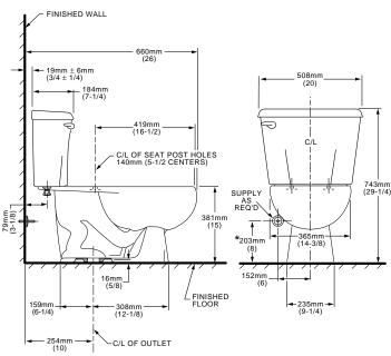
THIS COMBINATION IS DESIGNED TO ROUGH-IN AT A MINIMUM DIMENSION OF 254MM
