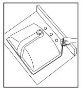
Carefully cut out the enclosed template, then position and trace the template on the countertop as shown on the template. Make a mark of the faucet hole centerline on the countertop. Drill a 1/2" pilot hole on the inside of the cut line. Use a saber saw or a keyhole saw to cut out the countertop opening.
