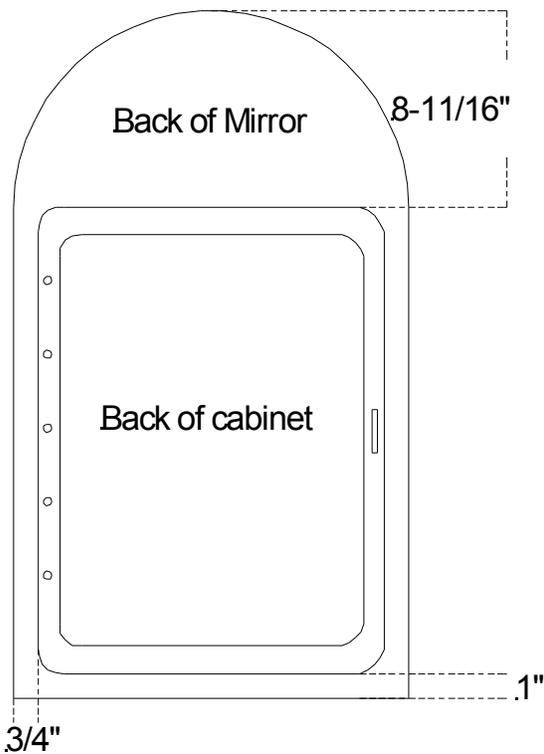
**96 Series Adjustable Shelf Cabinet(1A and 1B) Plastic(Polystyrene) Recessed or Surface Mounted**
