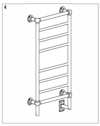
Unit must be wired to an on/off switch [not included] Make sure one is provided for installation.
