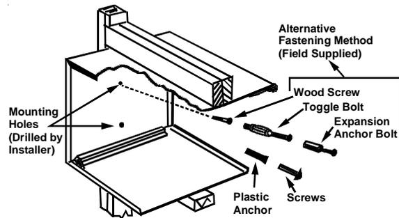
**Figure 10 - Wall Sleeve Attachment to Opening**
