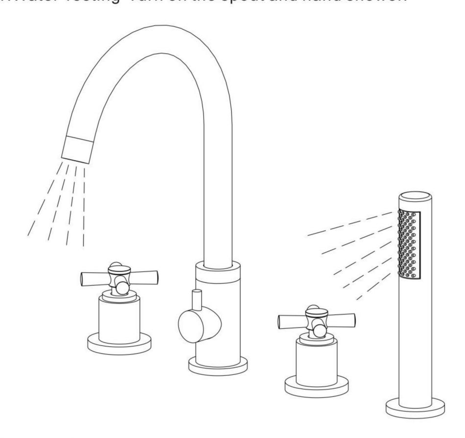
12. Turn off the spout and hand shower, and re-install the aerator. (Please ignore the step of re-install, if the model is without the aerator.)
